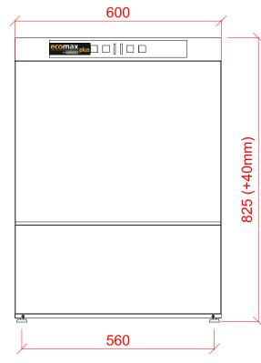
22mm CONNECTION VIA 2 METRE FLEXIBLE HOSE, FEMALE TERMINATION. WATER SUPPLY 10°C TO 60°C @ 0.6 TO 10.0 BAR MAX. INITIAL TANK FILL 10.6 LITRES. RINSE WATER USAGE 2.0 LITRES PER CYCLE. MAX USAGE 60 CYCLES PER HOUR.
