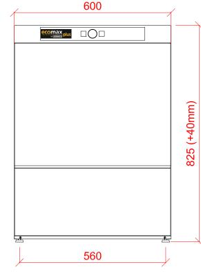
22mm CONNECTION VIA 2 METRE FLEXIBLE HOSE, FEMALE TERMINATION. WATER SUPPLY 10°C TO 60°C @ 0.6 TO 10.0 BAR MAX. INITIAL TANK FILL 10.6 LITRES. RINSE WATER USAGE 2.0 LITRES PER CYCLE. MAX USAGE 60 CYCLES PER HOUR.
